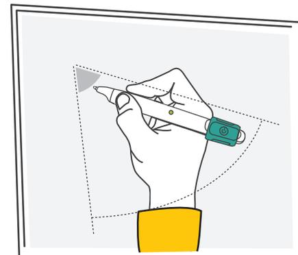
In order to have the Anoto Digital Pen working in a proper way on the wall, it is recommended to use it within an angle of 50 to 85 degrees.
